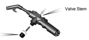
2.) Remove Wand Valve Nut by rotating counterclockwise. Press down on the exposed valve stem to remove the valve spring.
