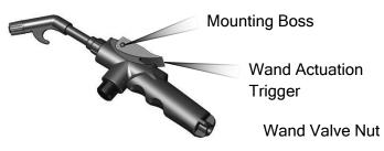
1.) Remove Wand Actuation Trigger Handle. Using a flat head screwdriver, carefully wedge the flat head between the wand actuation trigger handle and the wand body to separate from mounting bosses.
