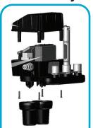
Install Batteries by **Removing Top Cover**
