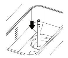
Remove and reinstall MIX FEED TUBE with inlet hole facing up (out of mix)
