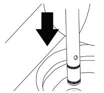
Install MIX FEED TUBE with inlet hole facing down (in to mix)
